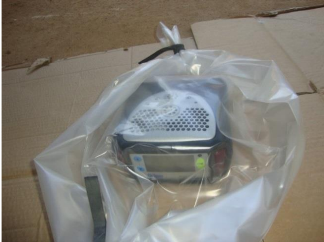
Figure 9: The device used for measuring content of methane placed inside a sampling bag
